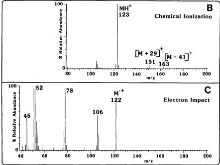
Figure 1. Total ion chromatogram (A) of extract of canned tomatoes recorded under GCMS conditions with mass spectral data of the peak as follows: (B) chemical ionization with methane as reagent gas, and (C) electron impact.
